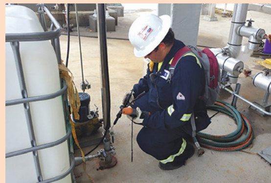
Vapour analysers and infrared cameras - just a few of the tools used for the downstream Fugitive Emission Management Program.
