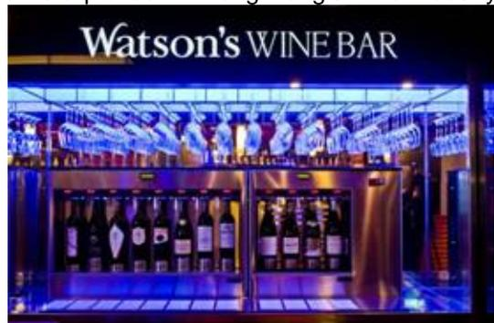
Watson's has utilised some of the latest technology from Italy in its new wine bar. Enomatic wine dispensing units are produced in Italy and are specially designed to keep wines under optimal conditions until they reach the glass. The Enomatic system allows guests the convenience of their own stored value card and simply swiping the card to choose from a range of premium wine.
